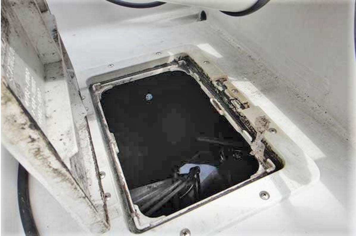
Poorly maintained or absent gaskets on hatches (even when new) can allow enough water into the bilge to overwhelm the pumps and sink the boat.
